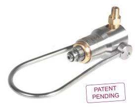
FasTest's G590 gas connector is simple to use with a no twist, no turn approach to filling. Simply connect onto your CGA 590 valve and lock into place with a forward movement of the bail handle roller actuator and you are ready to fill the cylinder in a matter of seconds.
