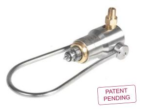
FasTest's G580 RPV gas connector is simple to use with a no twist, no turn approach to filling. Simply connect onto your CGA 580 RPV valve and lock into place with a forward movement of the bail handle roller actuator and you are ready to fill the inert gas cylinder in a matter of seconds.
