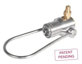
FasTest's G346 gas connector is simple to use with a no twist, no turn approach to filling. Simply connect onto your CGA 346 valve and lock into place with a forward movement of the bail handle roller actuator and you are filling the compressed air cylinder in a matter of seconds.
