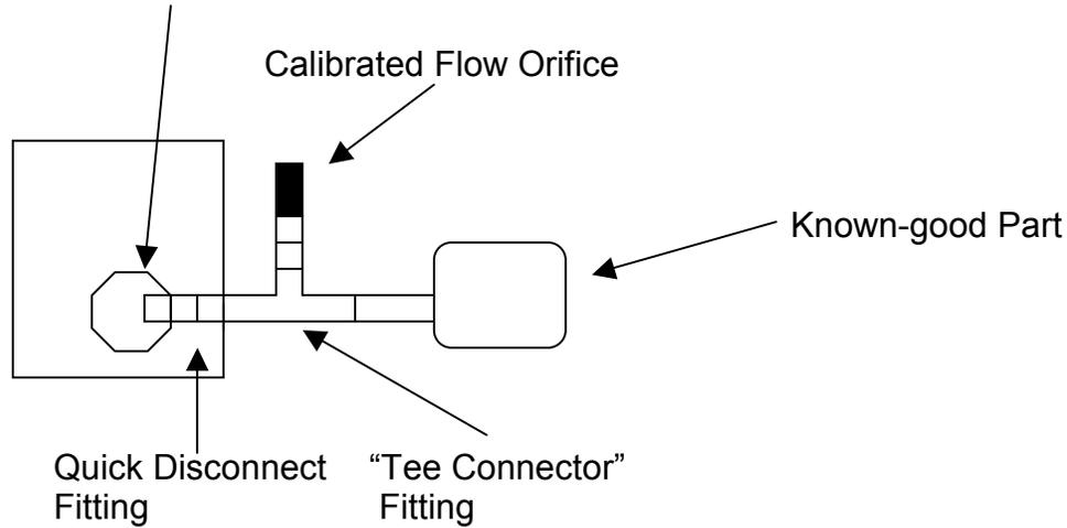
Use Dead End Plugs to cap off other ports if the instrument is a multi-port configuration.
