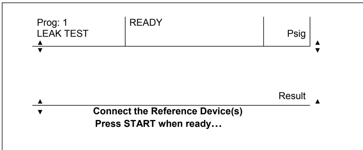
Prior to running any tests the operator must run a test on the memory device(s) in order to record the reference curve. When a reference device test is being run the Main screen indicates this as shown below:
