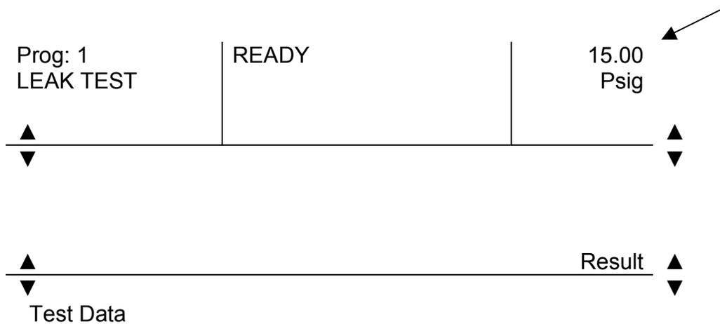
Touch the center of the screen to display the <Main> Screen. Touch the “Set Parameters” address and the <LEAK TEST> Screen is displayed.
