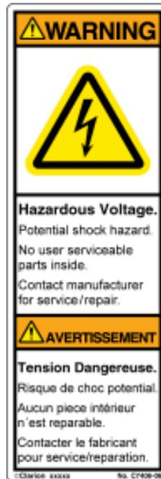
The hazard severity portion of this label warns the user of a potentially hazardous situation, which, if not avoided, could result in death or serious injury. The hazard is Hazardous Voltage. This voltage is inside the instrument
