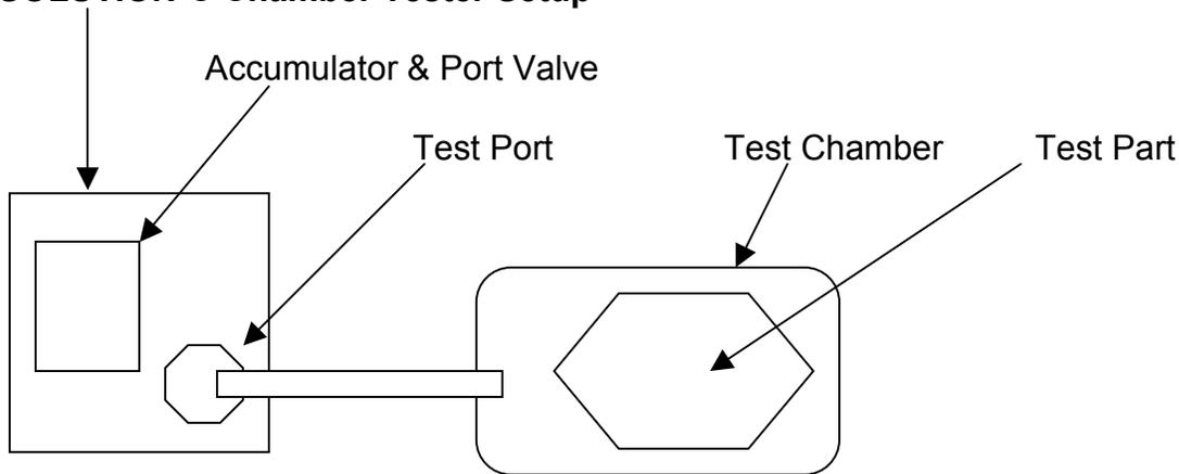
The volume of the Accumulator is designated  $V_A$  and during test setup it is pressurized to an initial pressure of  $P_A$ . The volume and test pressure of the empty test chamber are designated  $V_C$  and  $P_C$  and those of the test part are designated  $V_P$  and  $P_P$ .
