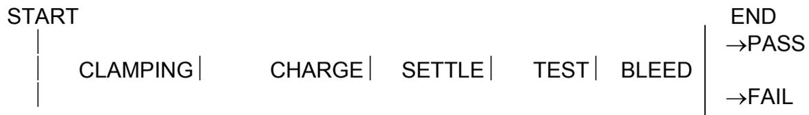
NOTE: When the bleed function is used the air inside the part flows back into the instrument carrying any loose debris or dust from inside the part. To prevent contamination of the internal pneumatics of the TME *SOLUTION* the use of a filter at the front port is recommended.
