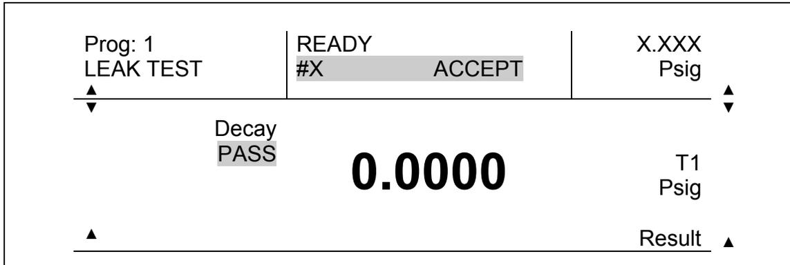
The test result may also be presented in a plot or decay curve format on the Main Screen Center as shown below
