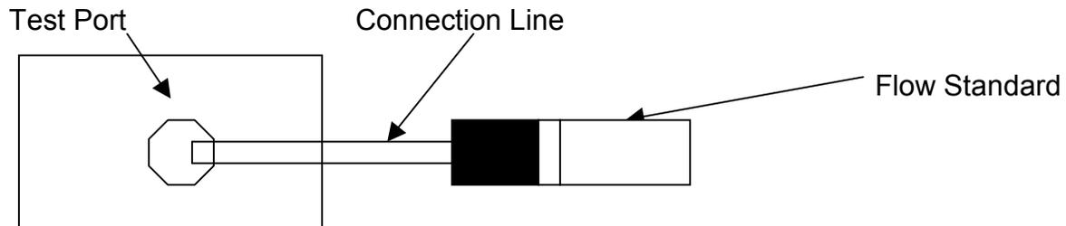
A Flow Reading will be displayed for instruments with Mass Flow Meters. Consult the Calibration Report for the expected Flow reading.
