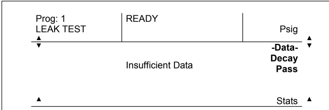
If the system is in the “Stats” Mode and there is sufficient statistical data in memory the test result is displayed as shown below.
