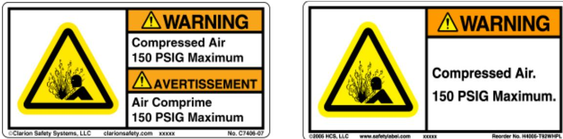
The hazard severity portion of this label warns the user of a potentially hazardous situation, which, if not avoided, could result in death or serious injury. The hazard is a compressed air input pressure above the instrument rated 150 PSIG Maximum.
