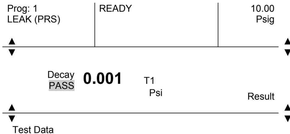
No calibration is required in the Pressure Decay Mode.
