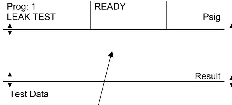
Touch the center of the MAIN SCREEN and the <Main Menu> Screen is displayed as shown below.
