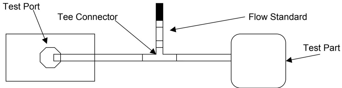
The test result will be a leak result on a good test part with a simulated leak rate equivalent to that of the flow standard. Consult the Calibration Report for the indicated leak rate.
