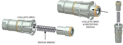
6. With piston down inside collets, hold collets closed with free hand.
