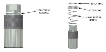
9. Using some type of arbor press or hand tool, press the snap ring into snap ring groove on body. Work press around snap ring until it snaps into groove. When snap ring is properly seated the stop ring will be inside sleeve.
