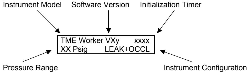
The display shows the Instrument Model Name, the Software Version, the Initialization timer countdown, the instrument Pressure Range and where applicable the Flow Range. The **ACCEPT**, **REJECT** and **TESTING** LED's are lit during the initialization period.
