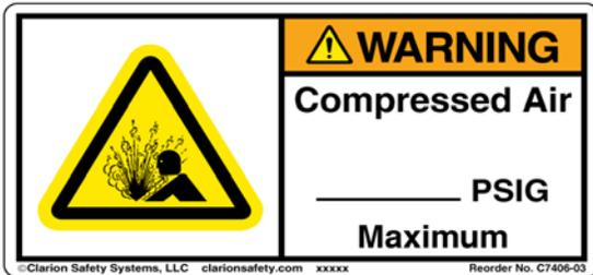
Custom instruments designed to have a compressed air input pressure above 300 PSIG Maximum will carry a Compressed Air Warning with the Maximum Compressed Air input pressure handwritten on the label.
