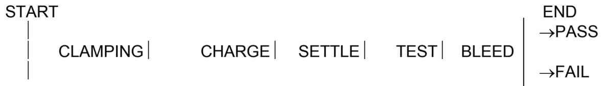
NOTE: When the bleed function is used the air inside the part flows back into the instrument carrying any loose debris or dust from inside the part. To prevent contamination of the internal pneumatics of the *WORKER* the use of a filter at the front port is recommended.
