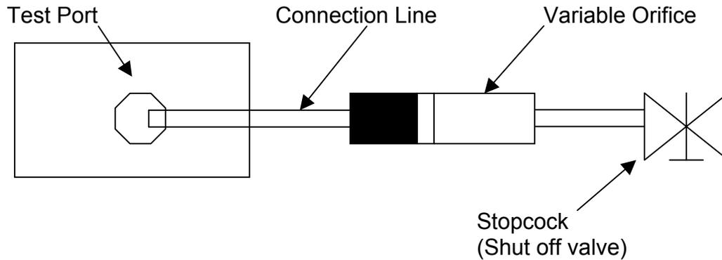
Connect the part to the test port. Verify that the stopcock is in the **closed** position.
