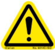
A black triangle with a black exclamation point on a yellow background is the ISO "General Warning Symbol". It is used to alert the user to a potential personal injury hazard. The general warning symbol can be used alone or in combination with a signal word to call attention to hazard information. Obey all safety messages that follow this symbol to avoid possible injury or death
