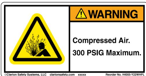
The hazard severity portion of this label warns the user of a potentially hazardous situation, which, if not avoided, could result in death or serious injury. The hazard is a compressed air input pressure above the instrument rated 300 PSIG Maximum.
