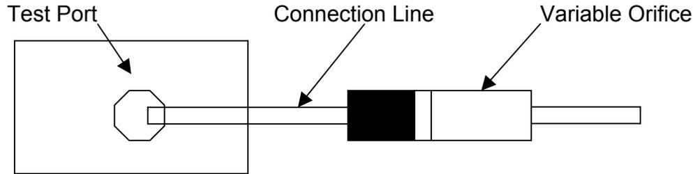
Connect the part to the test port. Verify that the leak orifice is in the **closed** position.
