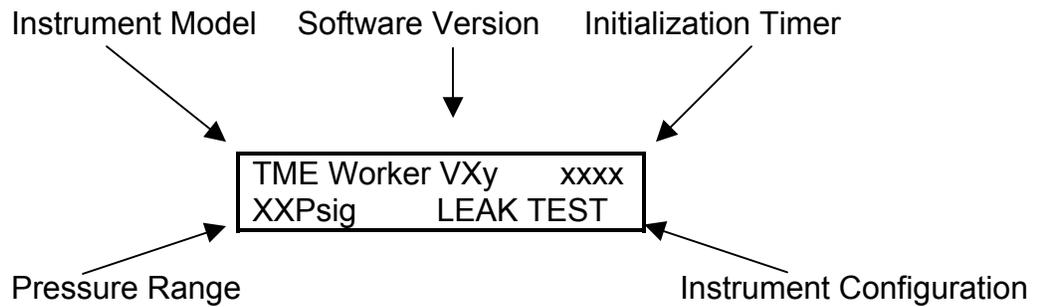
**LEAK AND FLOW TEST MODEL**
