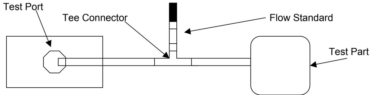
The test result will be a leak result on a known good part with a simulated leak rate equivalent to that of the orifice. Consult the Test Report for the indicated leak rate.
