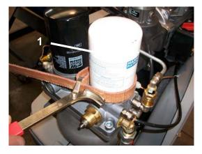
Replace the oil separator filter cartridge after the first 500 hours of use then every 2500 hours and in any event each time the oil is changed.
