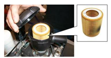
Remove the upper plastic shroud to gain access to inside the compressor.
