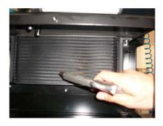
Remove upper and under plastic shrouds to gain access to inside the compressor.
