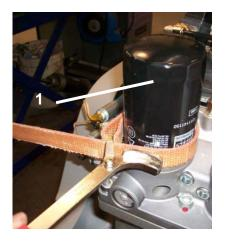
Replace the oil filter cartridge after the first 500 hours of use then every 2500 hours and in any event each time the oil is changed.
