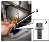
Once emptied, shut-off tap  ${\bf 3}$  and remove the attachment with tail piece.
