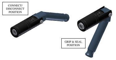
**Nulaws** JXL Connectors provide a reliable leak-tight connection that grips and seals straight tubing. Simply place the JXL connector onto a tube, activate the mechanical gripping and sealing action, then introduce the test media. For vacuum to 1000 psi applications with air, gas or liquid, **Fastest Nulaws** JXL Connectors provide secure, leak tight sealing.
