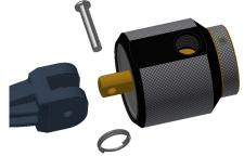
Using a small flat screwdriver or like tool, remove spiral retaining ring from body and discard.
