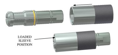
With sleeve loaded, stand connector up in vertical position and install new sleeve spring, stop, and new retaining ring. Using a pick or small flat screwdriver, push the retaining ring down body and into groove on body.
