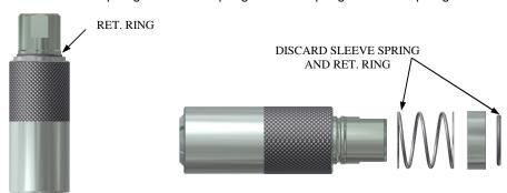
4. Remove sleeve in the same direction as retaining ring and sleeve spring. As sleeve is removed hold jaws collapsed with other hand. This will keep the piston contained inside the jaws.
