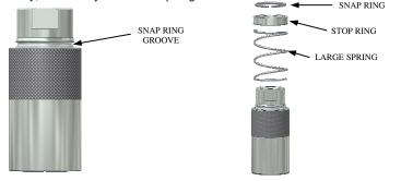
9. It's not required but using some type of arbor press will work the best to install the snap ring. Work the arbor press around snap ring until it snaps into groove. When snap ring is properly seated the stop ring will be inside sleeve.
